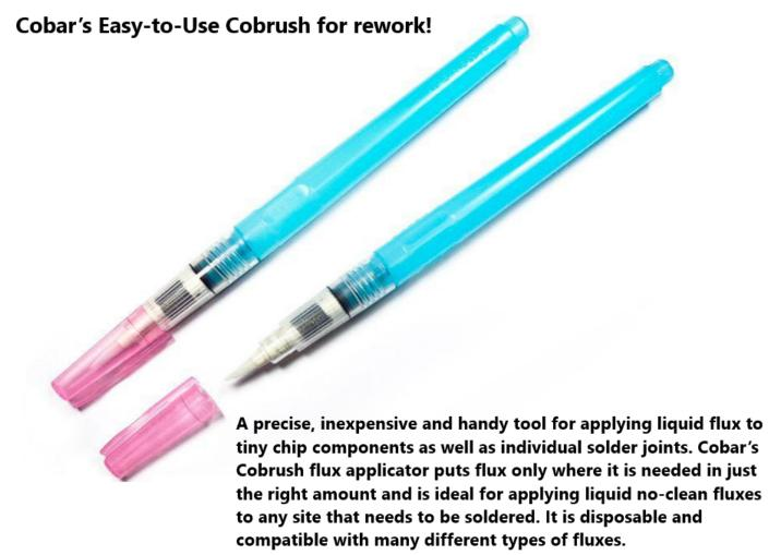
It's fine bristle tip allow the user to apply flux to very small areas in densely populated assemblies. The flux is dispensed by lightly squeezing the barrel, then using the gentle applicator bristles to apply the flux, just like an artist's brush, which allows the user to control the amount of flux flow.
